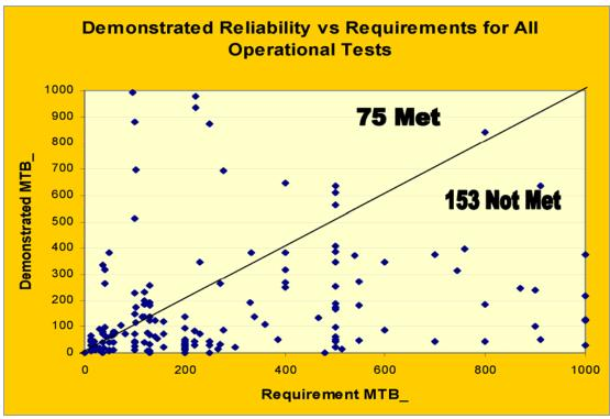
Figure 4: Army Systems Failing Reliability during Operational Testing (1997-2006).
