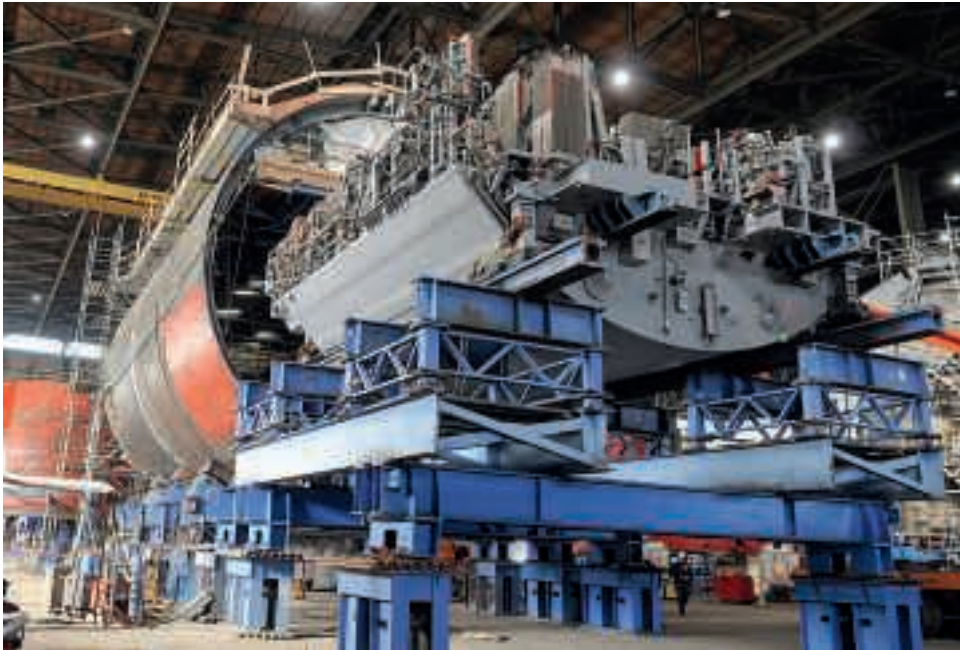
Module being inserted into the hull of a Virginia -class submarine. ( Navy Live blog )
