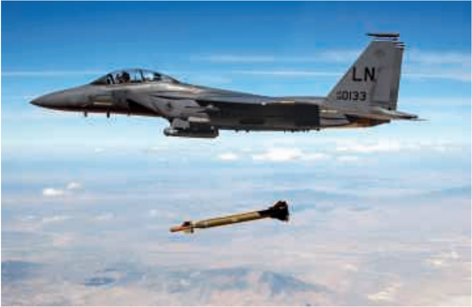
An F-15E Strike Eagle releases a GBU-28 "Bunker Buster." ( U.S. Air Force photo )
