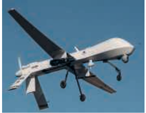
Predator UAV with a Hellfire air-to-ground missile mounted under the right wing. ( U.S. Air Force Fact Sheet )
