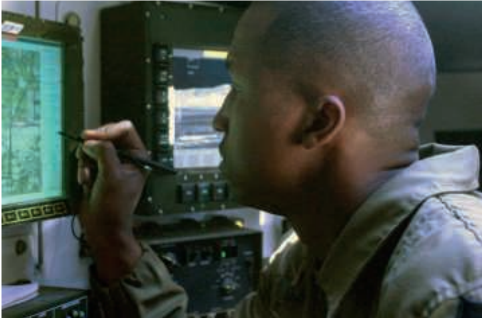
During an exercise at the National Training Center, Sergeant First Class Kenneth R. Dawson, 3d Infantry Regiment, checks an FBCB2 flat panel display installed in the antitank guided missile vehicle he commands. ( DIMOC )
