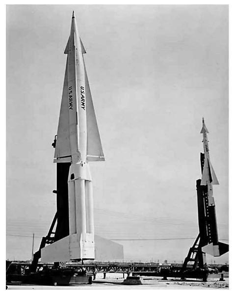
Nike Hercules (left) and Nike Ajax surface-to-air missiles on launchers. Courtesy, U.S. Army Aviation and Missile Life Cycle Management Command.
