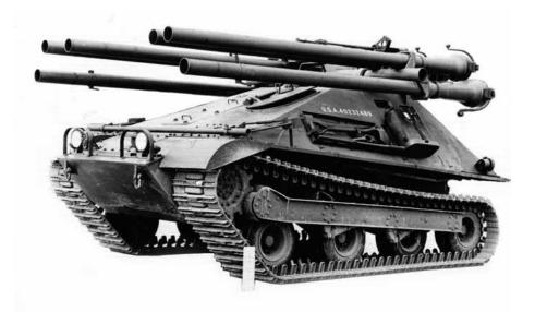
Pilot Ontos test vehicle mounting six 105-mm. recoilless rifles, 1952. (Note: In 1953, Ontos vehicles were modified to mount six 106-mm. recoilless rifles.)
