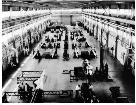
Nike Ajax missiles being assembled. Courtesy, U.S. Army Aviation and Missile Life Cycle Management Command.
