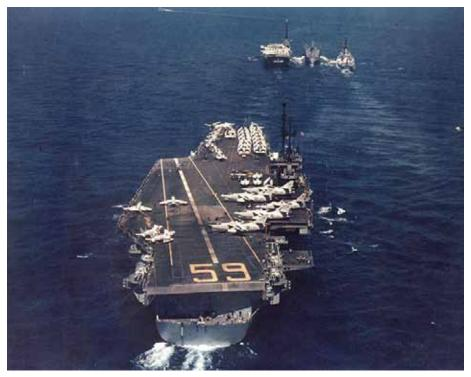
USS *Forrestal* (CVA–59) in Mediterranean Sea, April 1957. Note the angled deck and large size of the A3D Skywarriors (located on the starboard side of the ship, aft of the island superstructure) relative to the other aircraft.
