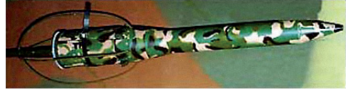
Air Delivered Seismic Intrusion Detector ( National Museum of the U.S. Air Force )
