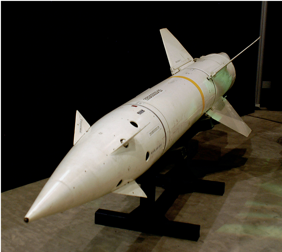
Martin AGM-12B Bullpup A on display at the National Museum of the U.S. Air Force. Bullpup A was armed with a 250-pound warhead. ( National Museum of the U.S. Air Force )
