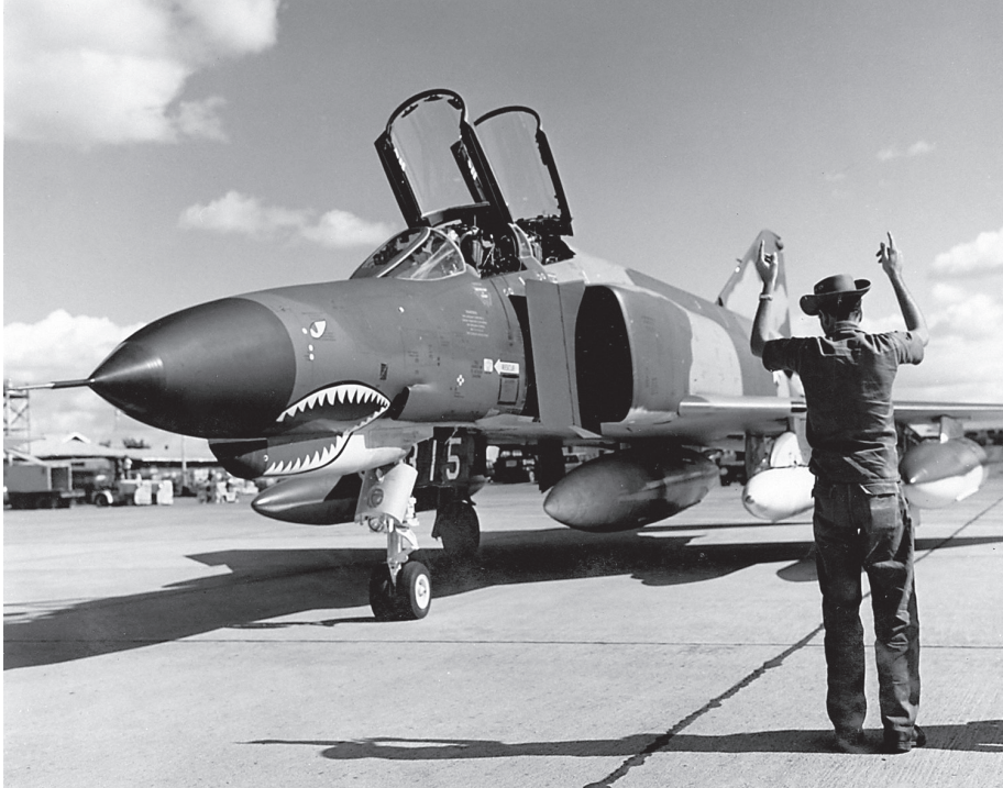
Among the F4-E's improvements over the F-4D was its 20mm gun. The first F-4Es arrived in Southeast Asia in late 1968. ( National Museum of the U.S. Air Force )
