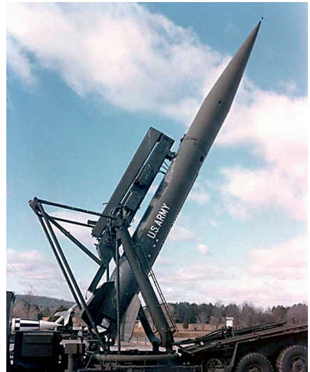
Sergeant surface-to-surface missile on launcher (U.S. Army Aviation and Missile Life Cycle Management Command)
