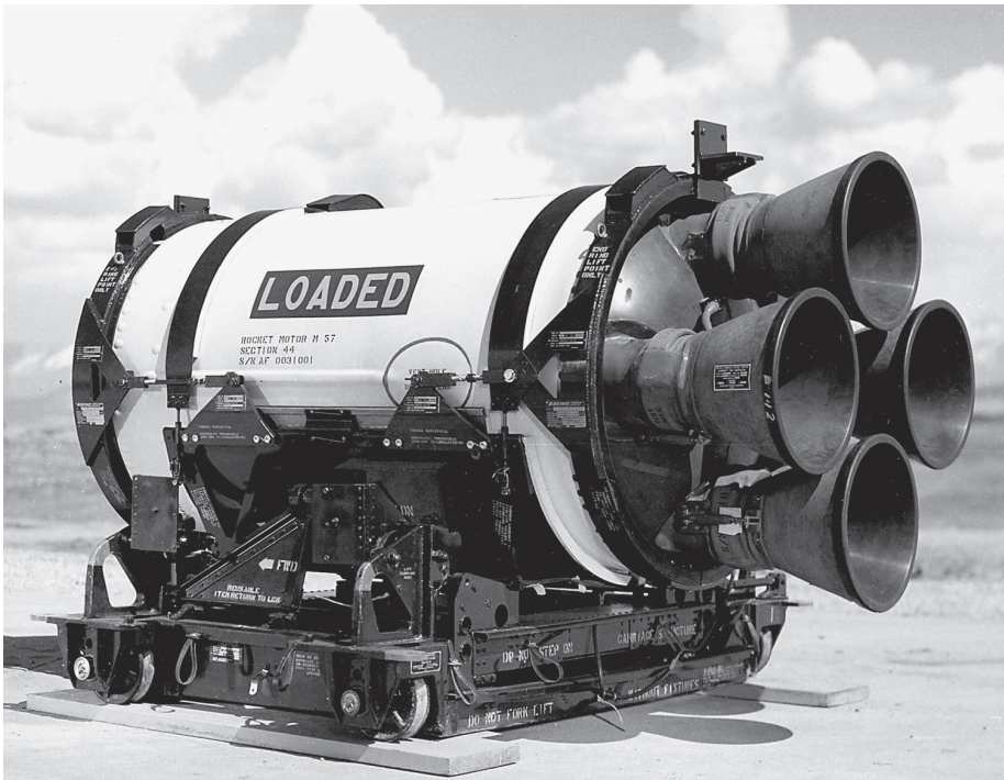
Each Minuteman solid-fuel engine stage contained four steerable rocket nozzles. This Minuteman I third-stage engine was made by Hercules Powder Company. ( National Museum of the U.S. Air Force )
