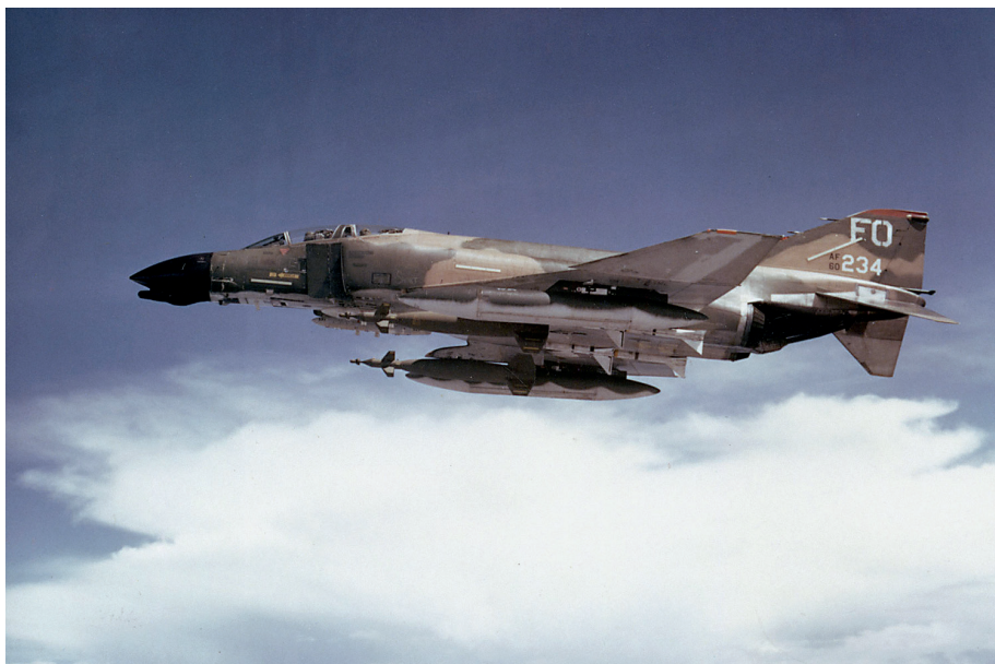
F-4D from the 435 th Tactical Fighter Squadron, 8 th Tactical Fighter Wing, armed with two Mark 84 laser-guided bombs (GBU-10 Paveway I) ( National Museum of the U.S. Air Force )
