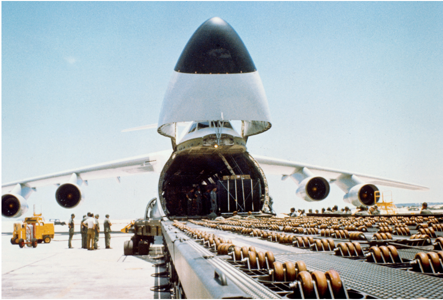
Front view of Lockheed C-5A Galaxy, visor raised, ready to receive cargo at Cam Ranh Bay Air Base, South Vietnam, September 1970 ( U.S. Air Force Air Mobility Command )
