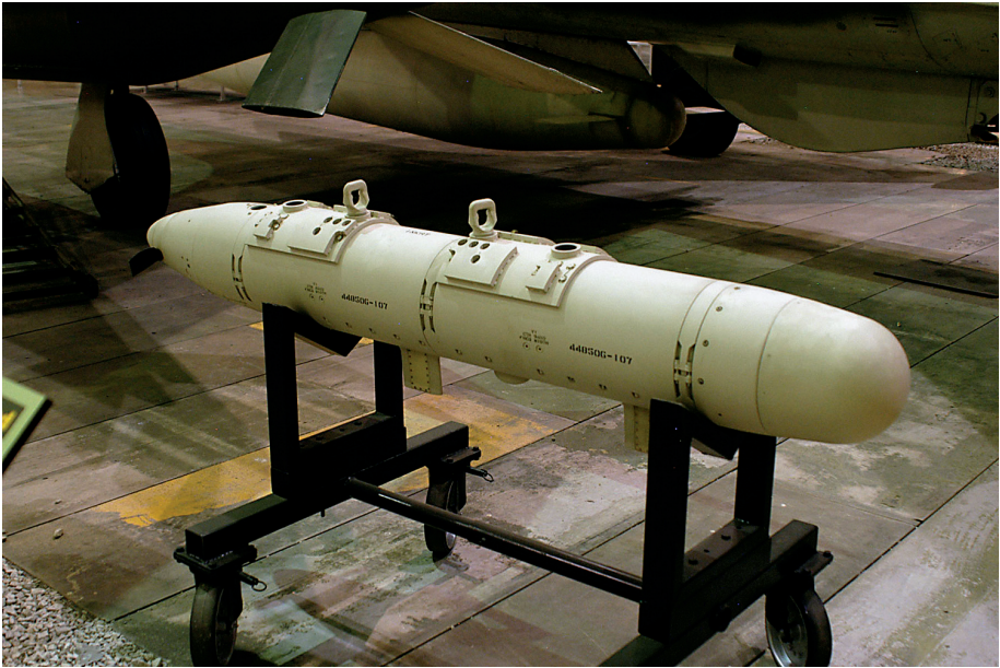
ALQ-71 electronic countermeasures pod on display at the National Museum of the U.S. Air Force ( National Museum of the U.S. Air Force )
