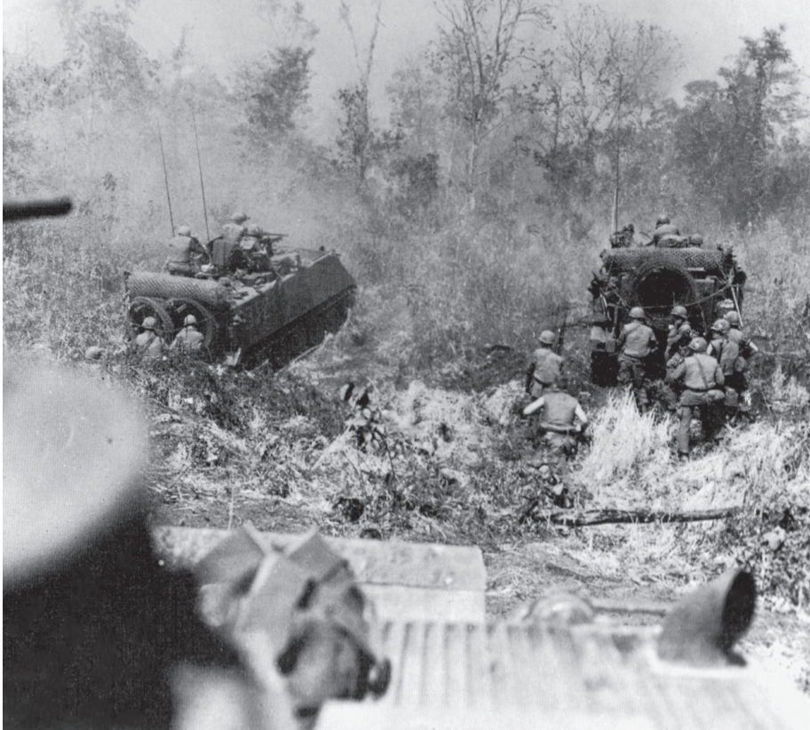
M113 armored personnel carriers clear the way during the Vietnam War ( U.S. Army Center of Military History )
