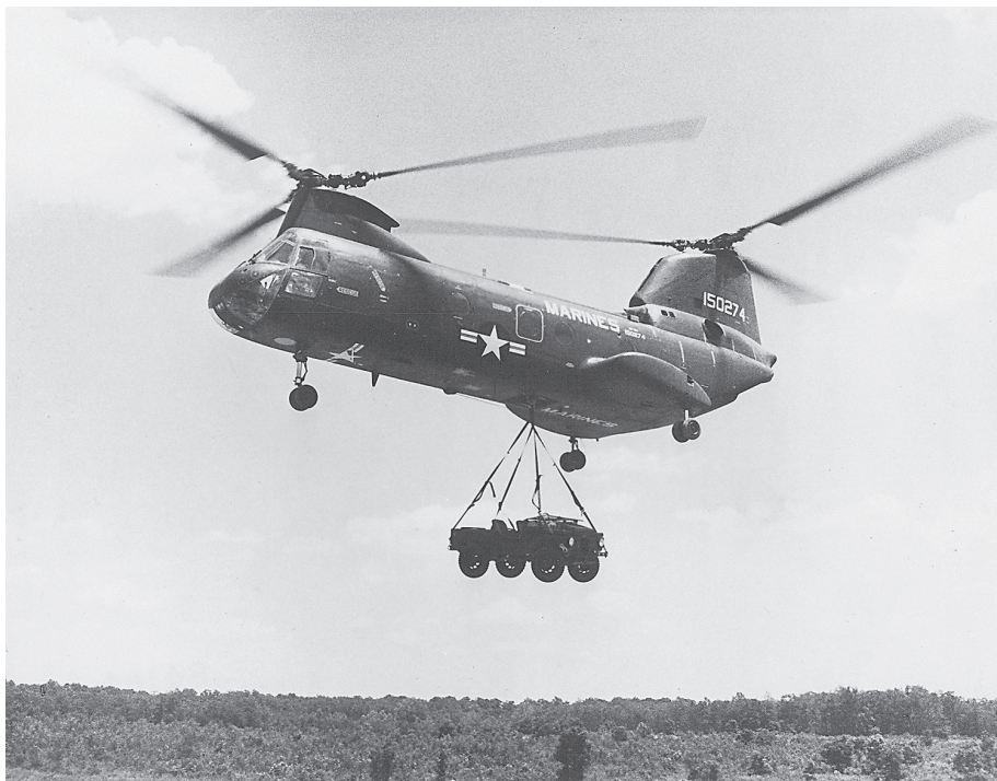
CH-46 Sea Knight lifts a 1,780-pound Mighty Mite vehicle on its 10,000-pound-capacity external cargo hook (U.S. Marine Corps)
