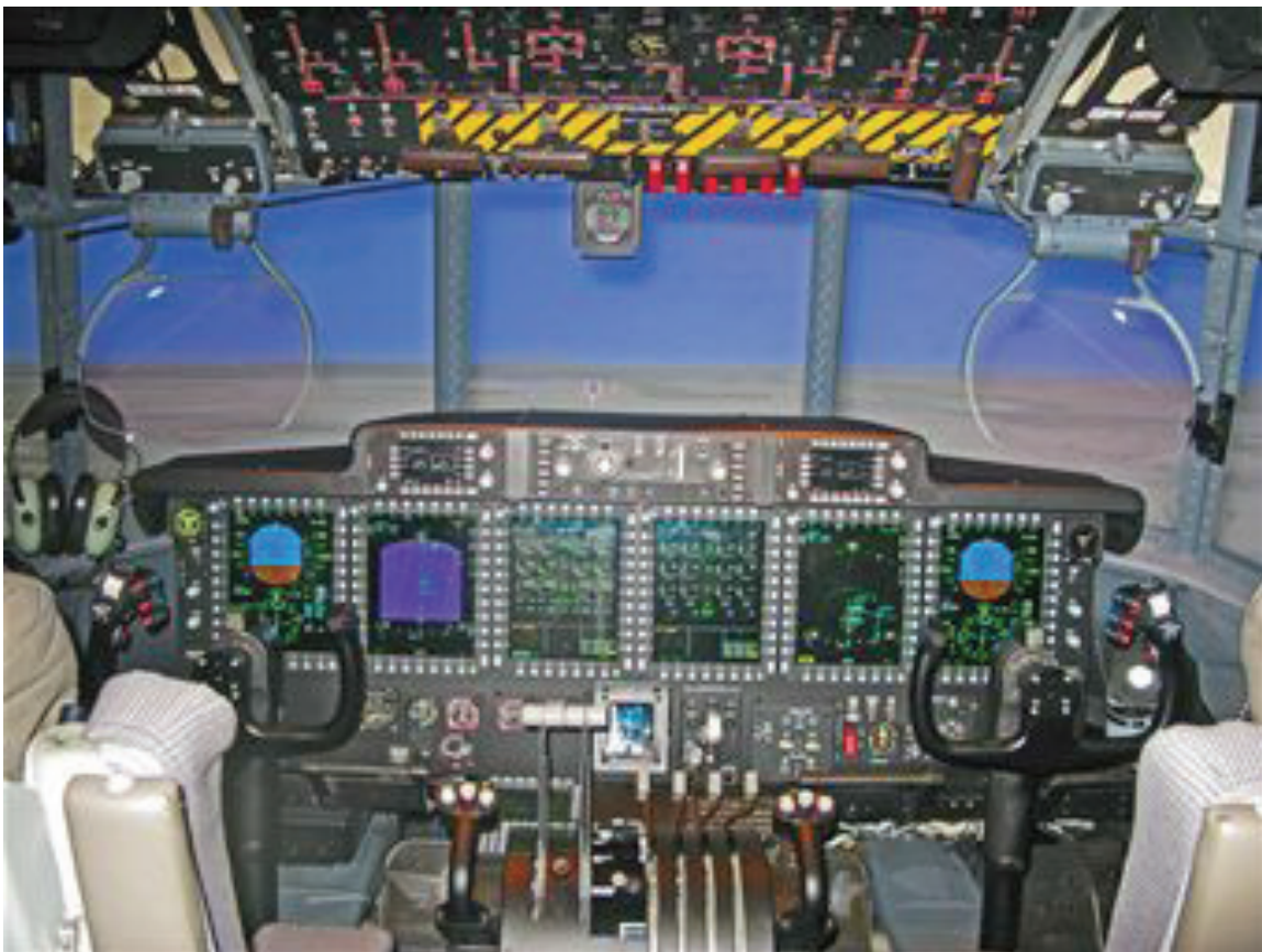
Figure 2.2. C-130 AMP Cockpit Simulator/Trainer Showing Cockpit Upgrades
