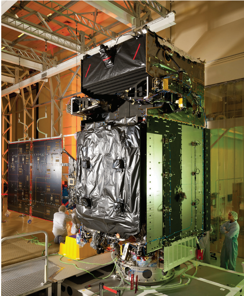
Figure 2.6. The Number Two SBIRS GEO Satellite Undergoing Ground Testing
